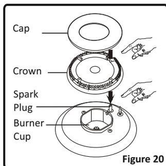
After the ignition, check the flames visually. If you see yellow tip, lifted or unstable flames; turn the gas flow off, and check the assembly of burner caps and crowns (Figure 20). Also, make sure that no liquid has flown into the burner cups. If the burner flame goes out accidentally, turn the burner off, ventilate the kitchen with fresh air, and do not attempt re-ignition for 90 sec.
