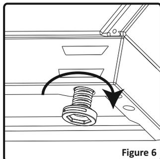
Your product stands on 4 adjustable feet. When the product is placed where to be used, check if the product is balanced. If it is not balanced, you can make the adjustment by turning the feet clockwise if required. It is possible to raise the appliance maximum 30mm by the feet. If the feet are adjusted appropriately, it is required not to move the appliance by dragging, it should be moved by lifting it up.
