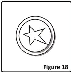
**Ignition by Spark Button:** Press the valve of the burner you want to operate and turn the valve in the counter-clockwise direction so that the knob is in maximum position and with your other hand, press the ignition button (Figure 18) at the same time. Press the ignition button immediately, because if you wait, a build up of gas may cause the flame to spread. Continue pressing the ignition button until you see a stable flame on the burner.
