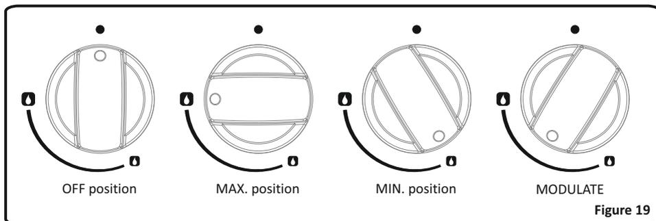
The knob has 3 positions: Off (0), maximum (big flame symbol) and minimum (small flame symbol). After you ignite the burner in maximum position; you can adjust the flame length between maximum and min. positions. Do not operate the burners when the knob position is between maximum and off positions.
